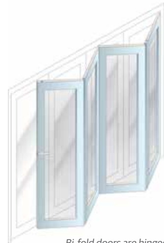
Bi-fold doors are hinged to fold neatly to one side in a concertina style.
